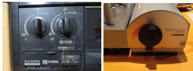
Figure 9: & 10: A built-in gas cooker control (left) and a portable gas cooker found in a Japanese Izakaya restaurant (right). To activate the built-in cooker, one has to push and turn the dial to the left. The portable cooker does not need to push but just turn left (photos by author).
