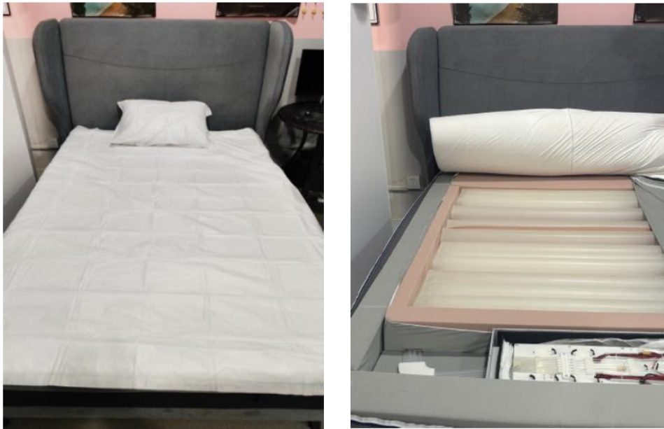
Figure 1: Experimental airbag bed (left) and internal structure (right).
