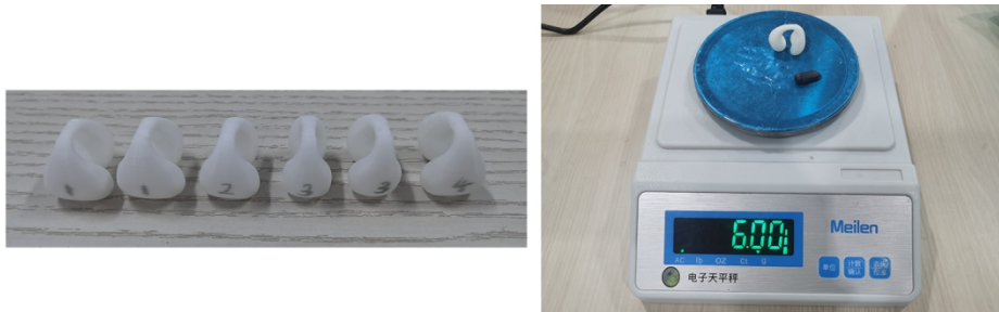
Figure 10: 3D printing of four prototypes (left), and earphone counterweight (right).
