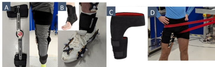
Figure 2: (A) Knee brace while walking in straight line, (B) ankle brace for single leg jump, (C) hip brace, (D) hip brace along with resistance band pulling the hip while performing sidewalk test.
