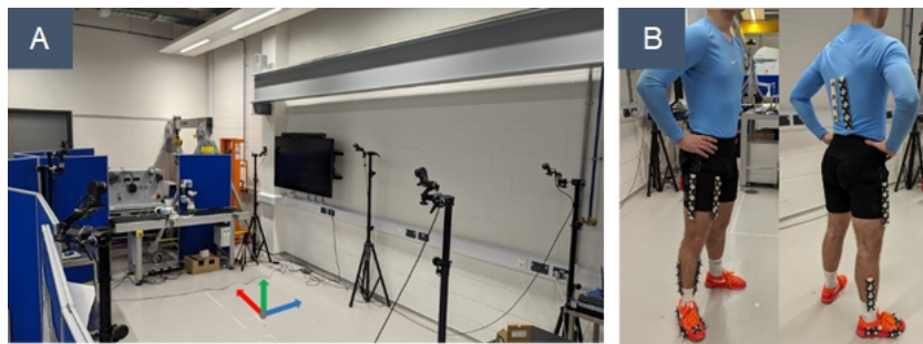
Figure 1: (A) OptiTrack system setup of 7 cameras used for testing. Axis orientation with x in red, y in green and z in blue. (B) Marker placements attached to the participants during the test.
