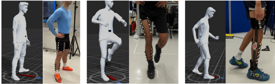
Figure 7: Real time data streaming from OptiTrack to Unity 3D. Integrating rigid body motion of the aligned anatomical frames into dynamic 3D animation.
