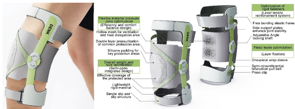
Figure 8: Optimized design solution for the knee brace.
