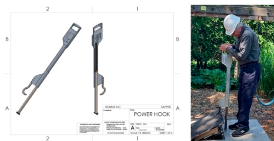
Figure 5: Left: CAD drawing of the battery-powered manhole tool, dubbed the “power hook”. Right: Power hook prototype lifting a simulated manhole cover. Note that the tool allows a worker to stand in an upright posture and exert minimal force to lift the cover from its rim (Marklin et al. , 2024).
