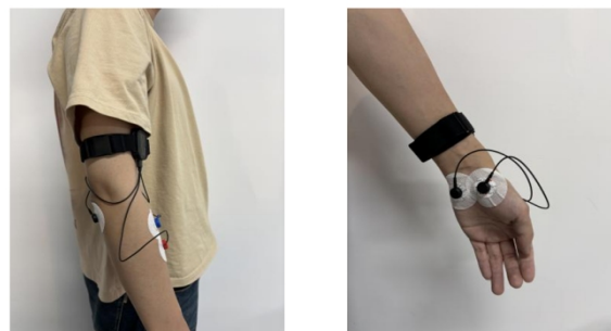
Figure 4: Schematic of a participant affixing myoelectric and electrodermal electrode pads and wearing a signal receiver.
