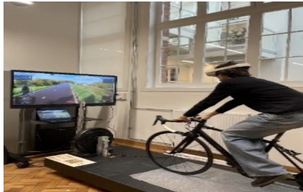
Figure 1: Participant using the cycling simulator, which replicates outdoor riding conditions through video, VR, audio, and dynamic resistance adjustments.
