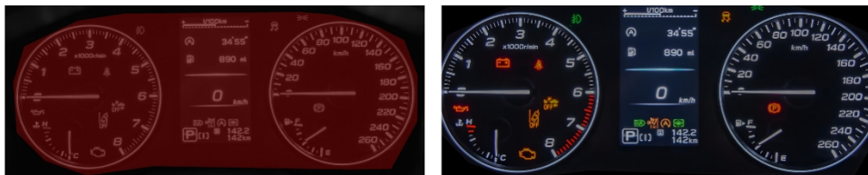
Figure 4: An example of processing a dashboard image. Left: the mask of cutting of images. Right: the materials after cutting and adding the black background.
