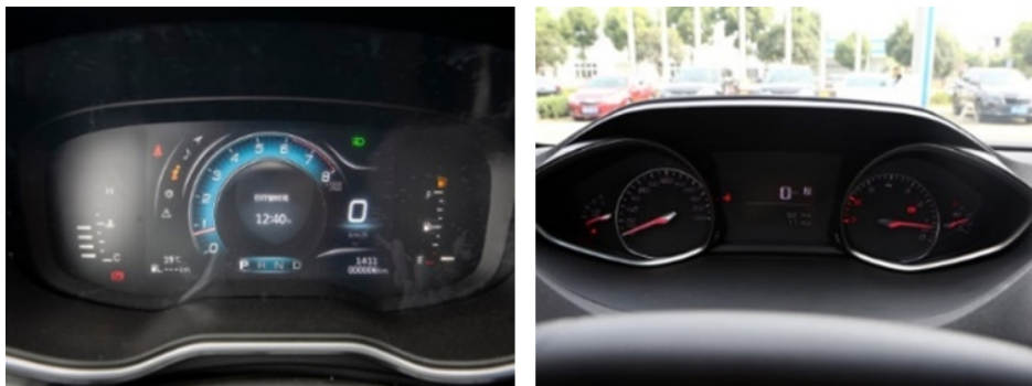
Figure 2: Example of the issues with raw images. Left: too much reflection. Right: distinct dash-board shape.
