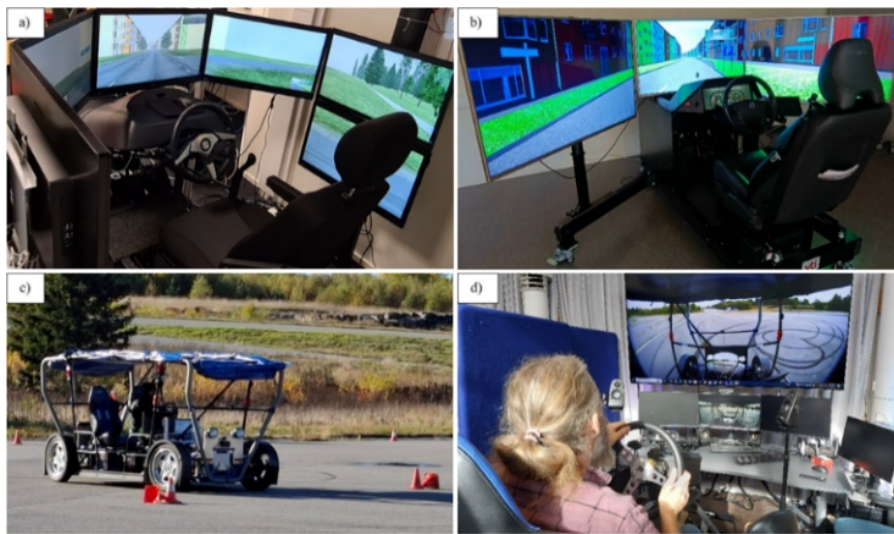
Figure 1: The apparatus used for the different experiments. The simulator used in experiments one and two (a). The simulator used in experiment three (b). The ROV (c) and the remote operation station (d) used in experiment four.
