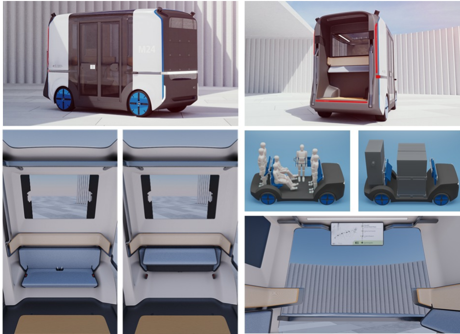
Figure 5: UMV Dualmover concept for combined transport of people and good with an adaptable interior (source: DLR).
