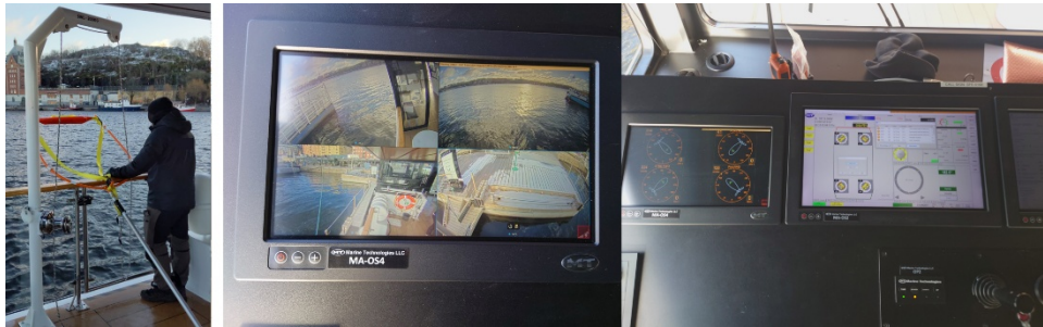
Figure 2: Rescue sling, on the left. Video feed panel, in the middle. Thruster control panel, on the right.
