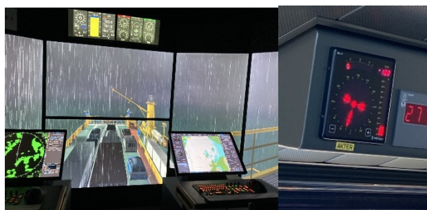
Figure 4: Left: simulation of scenario 2 with low visibility and heavy rain making navigation difficult and the radar unreliable. Right: rudder angle display onboard Tellus.
