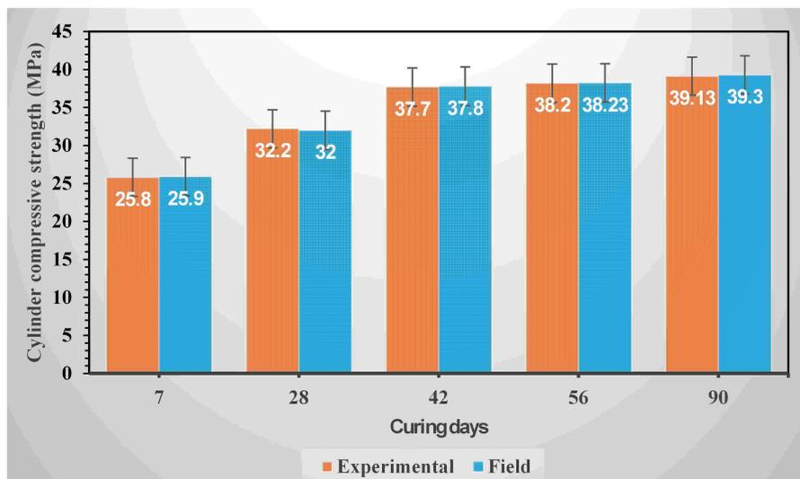
**Figure 5:** Compressive strength for cylinders.
