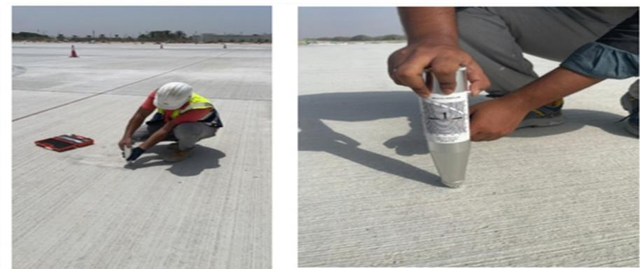
**Figure 2:** Rebound hammer test.
