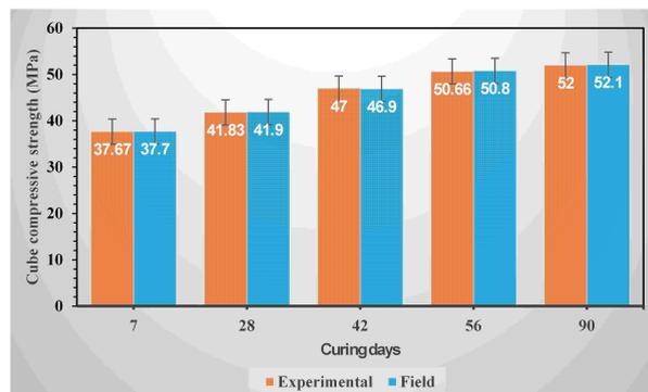
**Figure 4:** Compressive strength for cubes (MPa).
