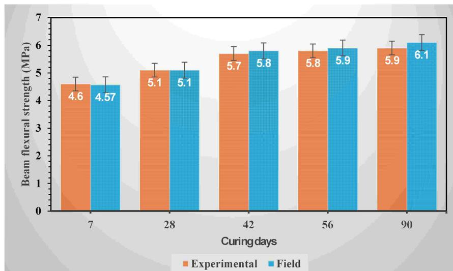
**Figure 6:** Flexural strength for beams (MPa).
