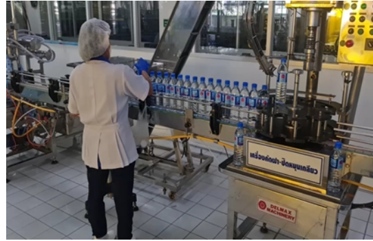
Figure 1: Operator closes the bottle cap by hand.
