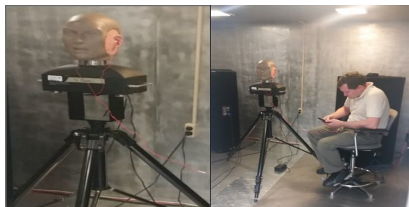
Figure 2: GRAS 45CB Acoustic Test Fixture (ATF) and testing lab setting during data collection.
