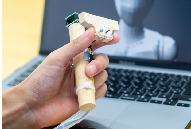
Figure 2: Prototype of the marionette-inspired controller, consisting of a handle, rotary encoder, and acceleration sensor.
