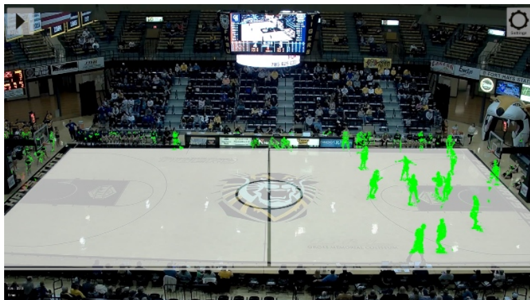
Figure 2: The live video feed is placed under the virtual court and made transparent for alignment and calibration purposes. The players are covered by green screen compatible pixels as defined in the foreground subtraction and contour processing.
