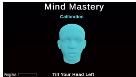
Figure 3: Gyroscopic calibration screen that records and averages directional tilts to personalize control thresholds.
