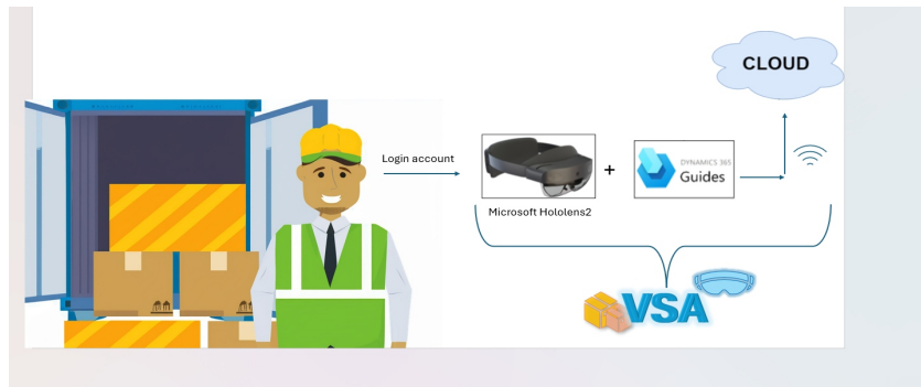
Figure 1: VSA architecture, including HoloLens 2 (hardware) and dynamics guides (software), with all digital information stored in cloud, accessible by powerful internet connection.
