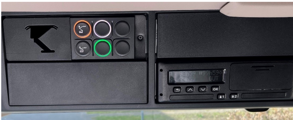
Figure 2: Pantograph control element of the BEE truck. Current status: system ready, pantograph retracted.
