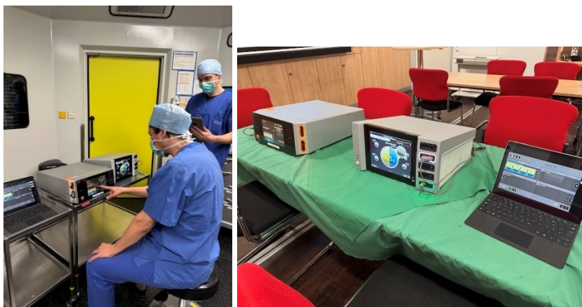
Figure 6: Setup for evaluation. Left: University Hospital Aachen's OR, HF devices are placed on two tables, right: University Hospital Essen's conference room, HF devices are placed on top of drape-covered tables.
