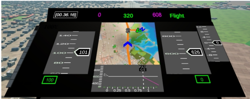
Figure 1: Cockpit interface display in the CAVE VR system showing the mini map and the glideslope display in the middle. The speed and altitude tapes are on the left and the right side, respectively.
