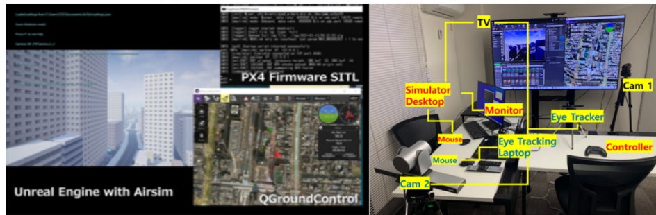
Figure 2: The structure of drone simulator apps and experiment environment with simulator, eye tracker and cameras (Maeng et al., 2024).
