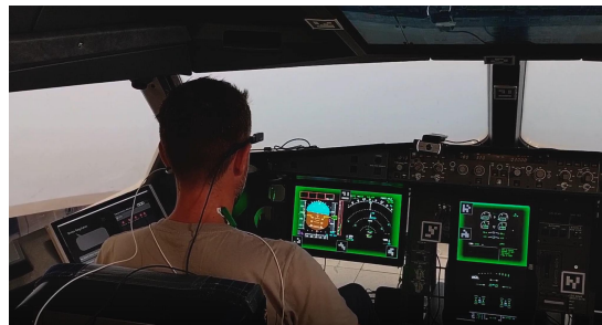
Figure 3: Illustration of FOCUS. The brightness of the screen borders (green rectangles) as well as the ambient colour of the cockpit is pulsating at the breathing frequency required for cardiac coherence, guiding the pilot to breathe at this optimal rhythm.
