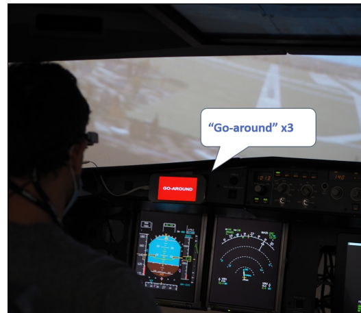
Figure 2: HARVIS assistant requesting a go-around due to abnormal flight parameters.
