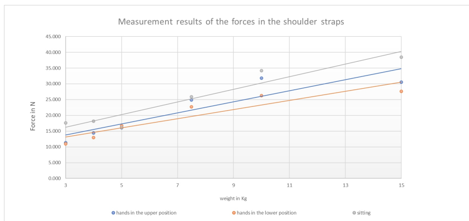
Figure 10: Measurement results of the forces in the shoulder straps.
