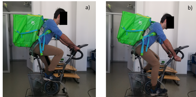
Figure 2: Handlebar positions: a) straight grip (hands up) b) low grip (hands down).
