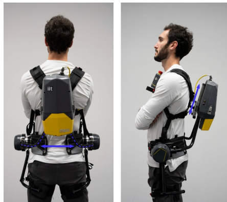
Figure 1: StreamEXO (Di Natali, 2024) including the compass design functional details for waist and hip widths and torso length adjustments.
