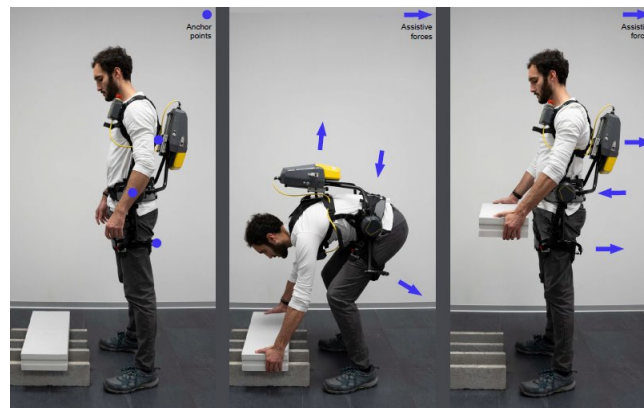
Figure 2: Anchor points of the exoskeleton (left) and trunk-leg force diagram generated by the exoskeleton.
