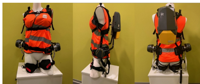
Figure 6: Female design ( beta ) of the exoskeleton harness on a manikin.
