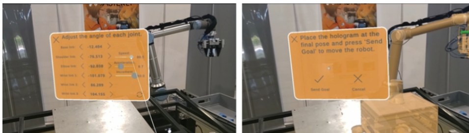
Figure 2: Two methods of manually programming the arm and gripper, using either specification of individual joint angles to adjust the arm’s position, or by virtually grasping and posing the arm in position.
