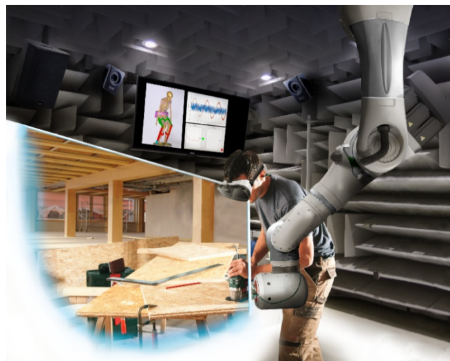
Figure 1: Vision of a testing environment for developing technical, symbiotic human-machine systems. A human is working with a virtual technical system in a testing environment. A robot with a real handle and a VR-environment gives him the feeling of a real-world task.
