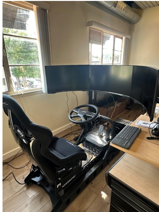
Figure 2: Physical layout of the SMART VR simulator station featuring three 32-inch wraparound displays providing 180° field of view, full-scale CMV cockpit with direct drive force-feedback steering wheel, professional pedal system, and ergonomically adjustable racing seat.
