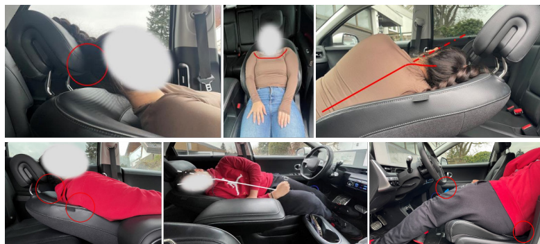
Figure 4: Limitations of current vehicle seats (here: Hyundai Ioniq 5) for reclined backrests in supine and lateral position.
