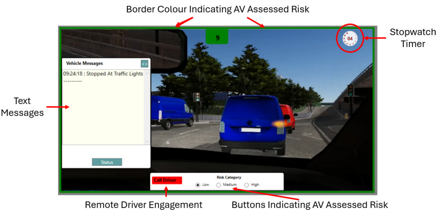
Figure 2: AV communication devices and remote driver engagement control.
