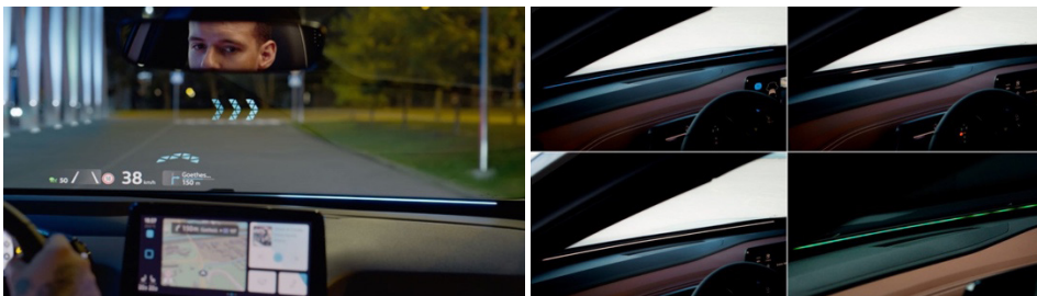
Figure 1: Ambient lighting display in Volkswagen ID3. Left: ambient navigation indicators. Right: lighting variations for different functions, such as charging status or VA feedback.
