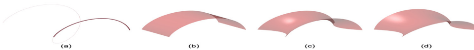
Figure 4: The evolution of basic parametric shapes: (a) half-periodic spiral curve; (b) lofted surface; (c) topological surface; (d) final optimized surface. (Source: the author).
