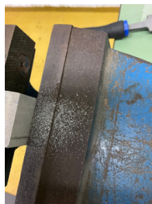
Figure 4: Material chips generated during the manual filing operation.
