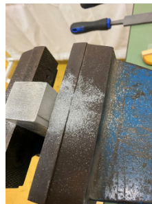
Figure 6: Material chips generated during the manual filing operation.
