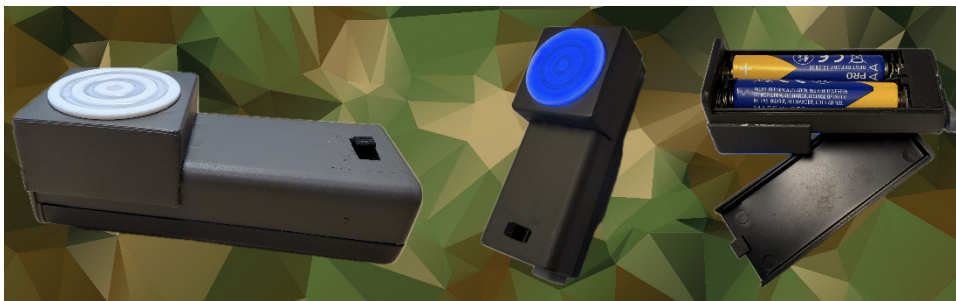
Figure 3: Prototype of the View2Decide system demonstrating the compact, wearable ESP32-based display module.
