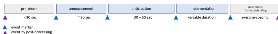
Figure 2: Stress-probe structure for comparable measurements in laboratory trials, field exercises and MR simulation. Short auditory-social probes are time-locked to biosignal windows, while longer stressor episodes support analysis of sustained stress and recovery (Paletta et al., 2025).
