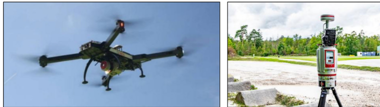
Figure 3: LiDAR mapping platforms which were used for collecting measurement data: Ricopter VUX-SYS (left) and Riegl VZ-400i (right).
