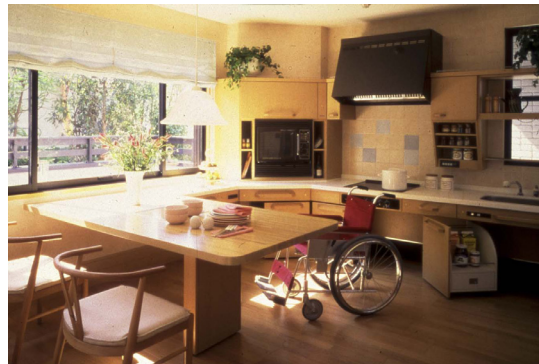
Figure 6: Counter kitchen set for wheelchair users.
