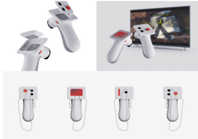
Figure 4: Modular interaction system and task-oriented reconfiguration.
