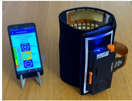
Figure 1: The ShefStim device, arm sleeve and mobile phone interface.
