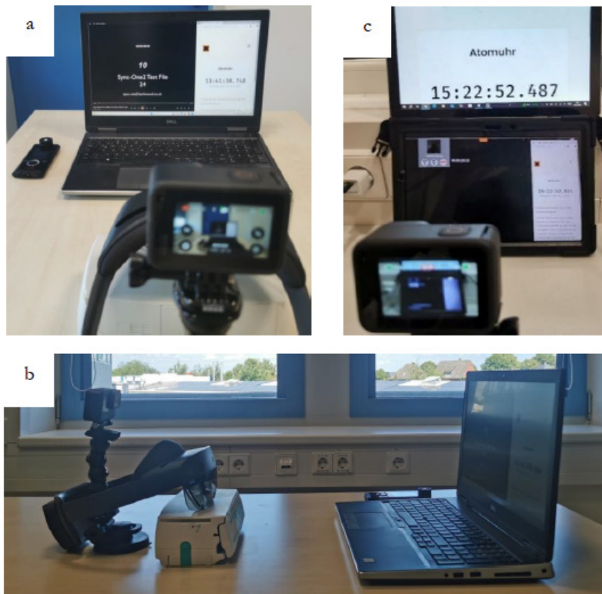
Figure 2: Experimental setup for measuring audio and video latency and audiovisual synchrony using synchronized light and tone makers and time alignment via web-based atomic clock.
