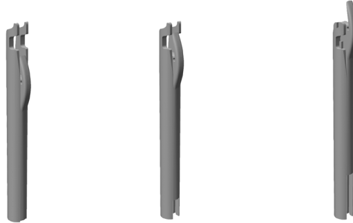
Figure 7: The three operational pin states: open, closed, and eject (left to right).
