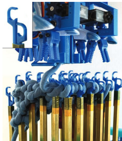
Figure 2: Motorised needle array used to actuate solid-knit loop transfers (Guimbretière et al., 2025).
