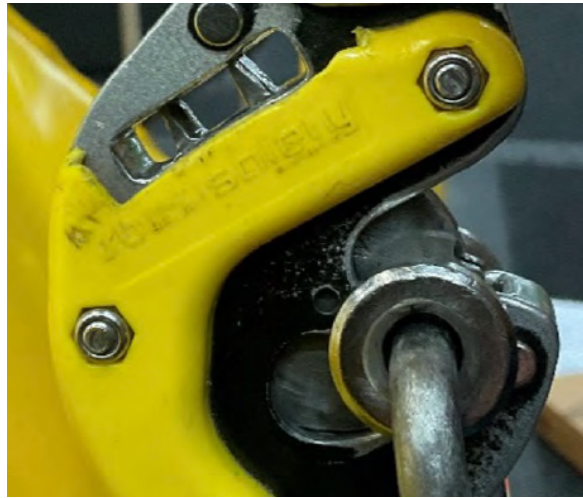
Figure 4: Side view of the heavily worn Self-Belay Body which failed depicting the locking key being able to be removed when the Self-Belay Maillon connector was not fully engaged (Eager, 2025).
