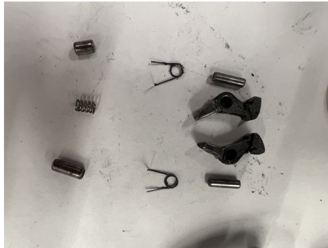
Figure 6: Self-Belay Body worn anchors and pins before they were cleaned, (Eager, 2023).
