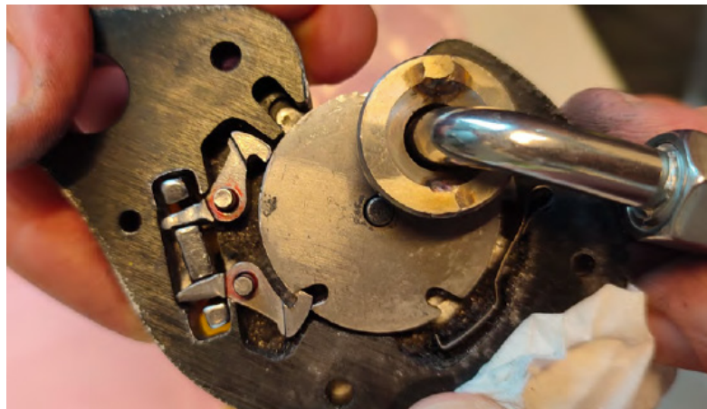
Figure 5: Disassembled and partially reassembled heavily worn Self-Belay Body which failed depicting a single locking anchors engaged within the worn Self-Belay Maillon connector partially engaged (Eager, 2025).
