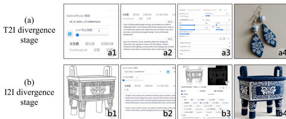
Figure 4: In the Text-to-Image (T2I) divergence stage, users can carry out the following steps: (a1) select the T2I function, (a2) enter the corresponding prompts, (a3) tweak the image generation parameters, and (a4) check the final generated outputs. In the Image-to-Image (I2I) iteration stage, the process involves: (b1) uploading a design sketch or reference picture, (b2) inputting specific prompts, (b3) adjusting the ControlNet configurations, and (b4) reviewing the generated image results.
