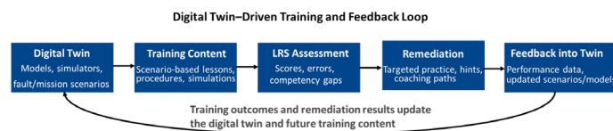
Figure 2: The enterprise feedback loop for training. Operational data flows back into the digital twin to generate new training scenarios, closing the loop between operations and workforce development.
