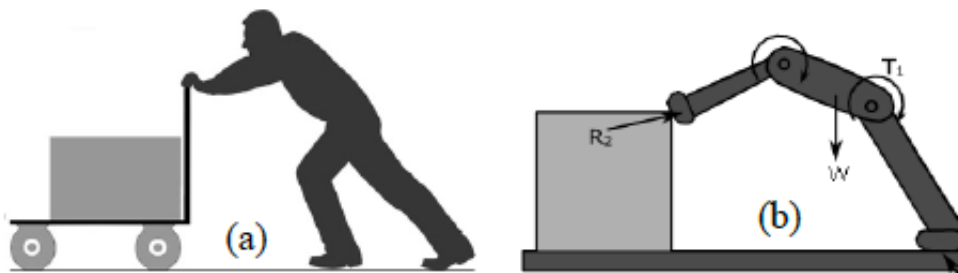
Figure 3: Cart pushing scenario (a) human posture (b) kinematic representation of posture.
