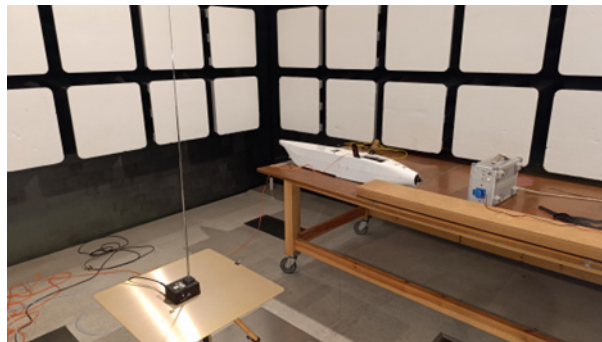
Figure 9: View of the SMS during measurement of the electric field strength placed in the enclosure in the frequency range from 10 kHz to 30 MHz with the V polarization of the measuring antenna.
