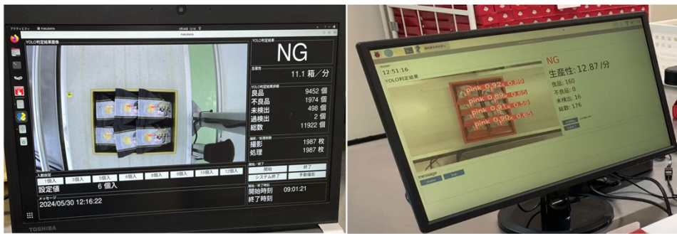
Figure 3: Continuous monitoring GUI for conveyor-line oxygen-indicator color evaluation.
