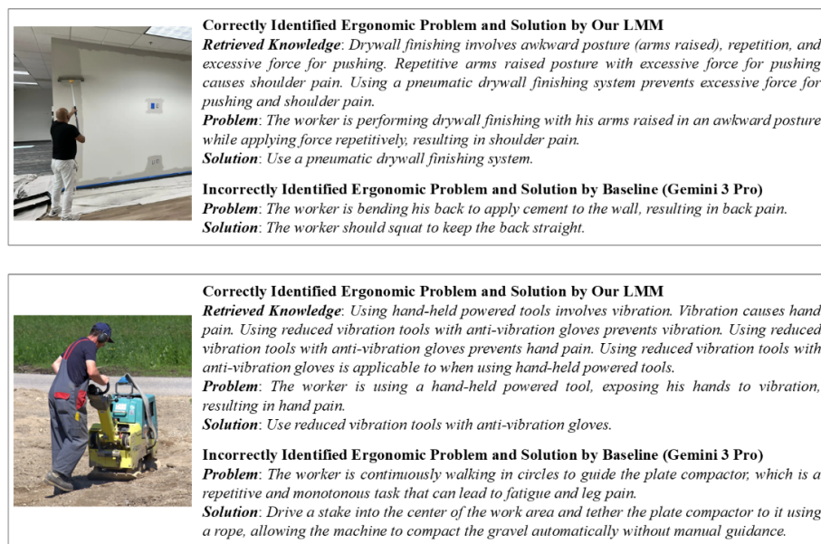
Figure 3: Correctly identified ergonomic problems and solutions by our LMM and incorrectly identified ergonomic problems and solutions by the baseline model (Gemini-3-Pro) (pxhere.com; finefinishescustompainting.com).
